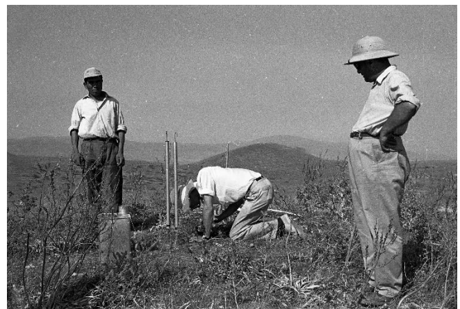
Figure 1. David Greenewalt (brother of director Crawford H. Greenewalt, jr) in 1961, surveying one of the Lydian tumuli with electrical resistivity, the first use of geophysics at Sardis. The survey failed to locate the burial chamber — in retrospect, not surprising since the mound is the size of the Great Pyramid in Giza while resistivity can penetrate to a depth of only a few meters. Prof. Hanfmann followed this with a three-year campaign of tunneling within the mound.
