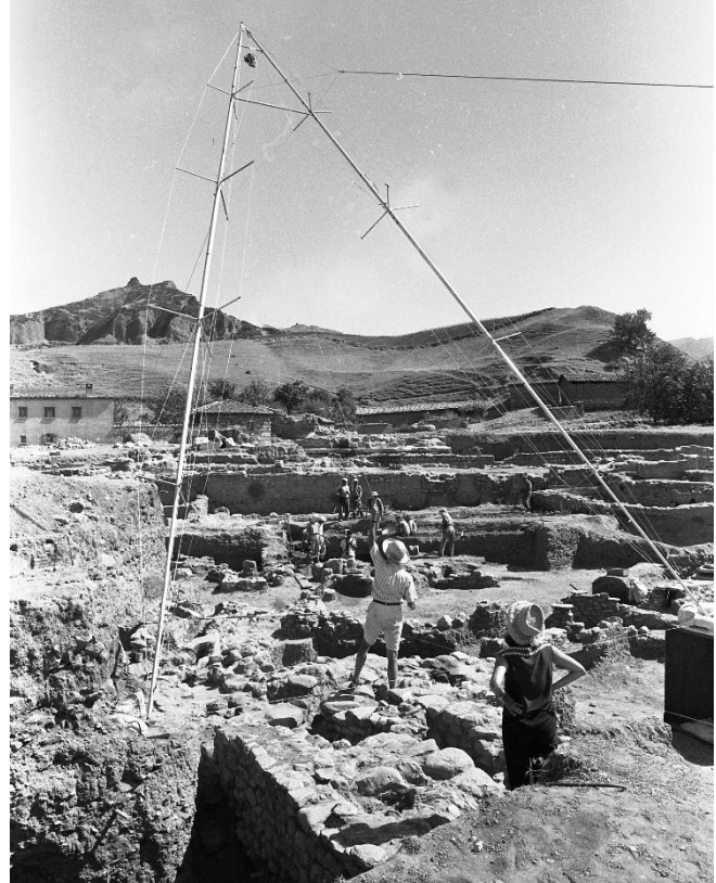
Figure 3. The Whittlesey Bipod, invented to take aerial stereo photographs of excavations trenches, in use in 1964 at sector PN. The Bipod was far more controllable than balloon or kite photography, and could be rectified on film to produce stereometric photos and three-dimensional representations. Today we use drones and photogrammetric software for the same purposes (fig. 6).
