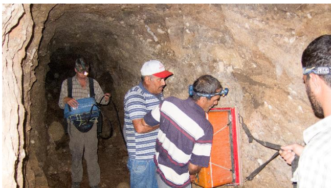
Figure 2. Geophysicists Stefan Giese and Christian Hübner of GGH Solutions in Geoscience surveying the same tumulus in 2011 using ground-penetrating radar from within tunnels dug in the 1960s. The team used electrical resistivity, electrical resistivity tomography, magnetometry, and GPR. Although they identified an anomaly, further tunneling showed that these were not the chamber, and despite digging almost half a kilometer of tunnels within the mound, the burial chamber remains undiscovered.
